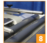
Horizontal self centering guides for simple case size setup
