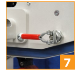
Selectable floating upper head processes compressible overfills
