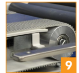
Self-tensioning & self-tracking drive belts simplify belt replacement
