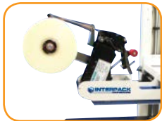
Tip up top tape head eases roll replacement
