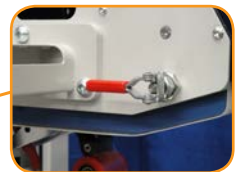
Selectable floating upper head processes compressible overfills
