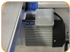
One ½ HP gear motor to process up to 85 lb cases
